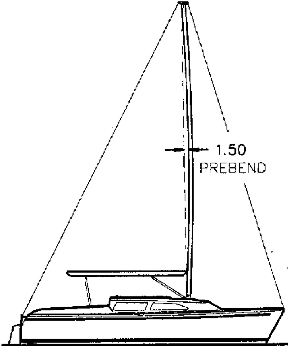
NOTE: Rigging tensions may be measured with LOOS & Co. Model B tension gauge.
